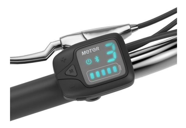
LD801 display is simple and beautiful as it adopts the scientific ergonomic curve design. The LED is not only clearly visible in the sunlight but also displayed with soft light under the night mode that makes riding safety.
